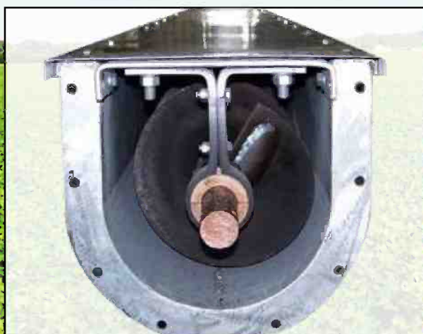
226 Style Hanger bearings with insert options of wood, nylon or UHMW. Made for your specific application.
