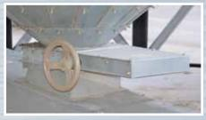
The hopper's discharge opening may be equipped with heavy-duty rack and pinion or roller-style unloading gates.
